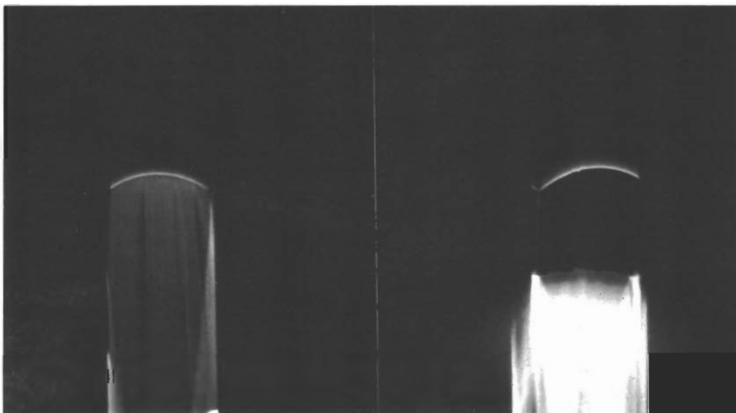
Fig. 8 RMC trace of detonations emerging from charges of RDX at 60% of crystal density. The charge on the left is at 580 torr while that at right is at a few microns.
